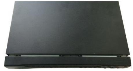
⑥ Put the cover in accordance with the clip and then place the upper cover back. Secure the screws in the rear panel and the side panel.
