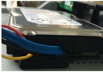
⑤ Connect the HDD cable and power cable.
