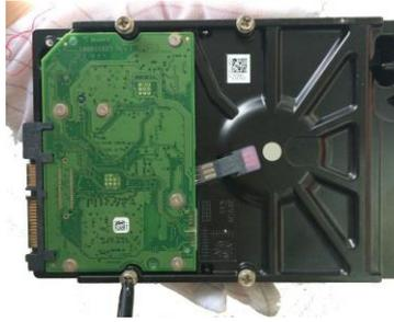
② Fix four screws in the HDD (Turn just three rounds).
